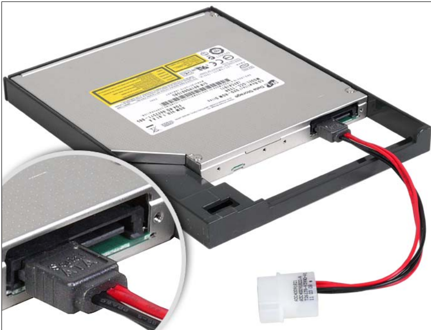
Figure 34: Connecting the PS adapter cable to the DVD drive
